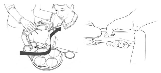
When the Teach Icon is covered, the Arm will be free for the Caregiver to move. The last two sections of the Arm will remain engaged and will keep the Spoon level when moving within the teach space. If resistance to movement is present, the thumb is probably not completely covering the Teach Icon. DO NOT FORCE the Arm to move as this may cause motor damage.
