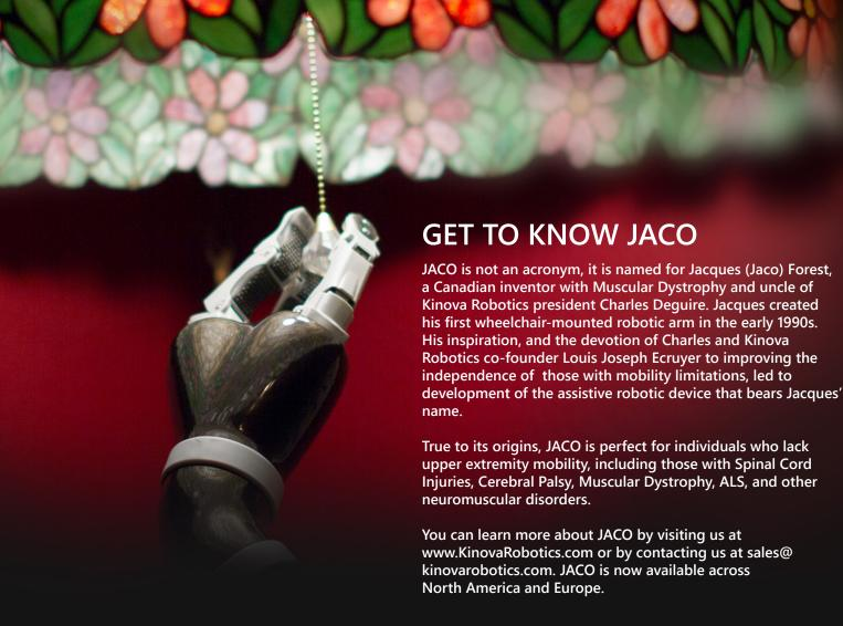
JACO can lift two pounds fully extended and up to three pounds maximum while providing six-degrees of motion. This means you can manipulate JACO to approach objects from almost any angle, such as picking up an object from the floor or reaching up into a cabinet.
